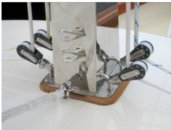
Plain bearing blocks fitted at the mast base
