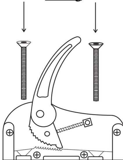
Use 6mm (1/4") Counter sunk stainless steel fastening, full nuts and penny washers to secure
