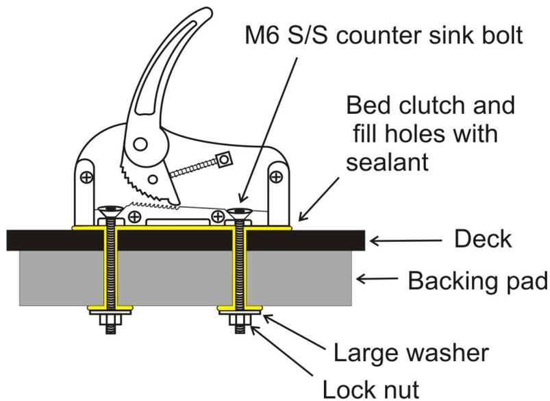
To ensure the best watertight seal is achieved, we would recommend slightly tightening the bolts, allow the sealant to cure for 24 hours and then tighten the bolts fully. This will allow the sealant to form a watertight gasket.
