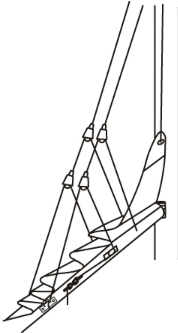
The lightweight Lazy Jack System allows the mainsail to be easily reefed or stowed in all weather conditions.
