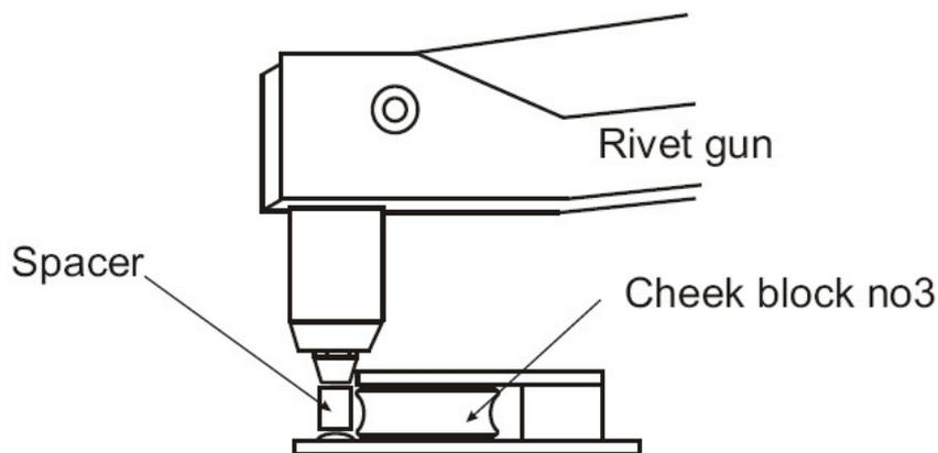
When riveting the cheek block there is a limited space for the rivet gun so use the brass spacer between the rivet gun nozzle and the cheek block to ensure the rivet is correctly aligned.
