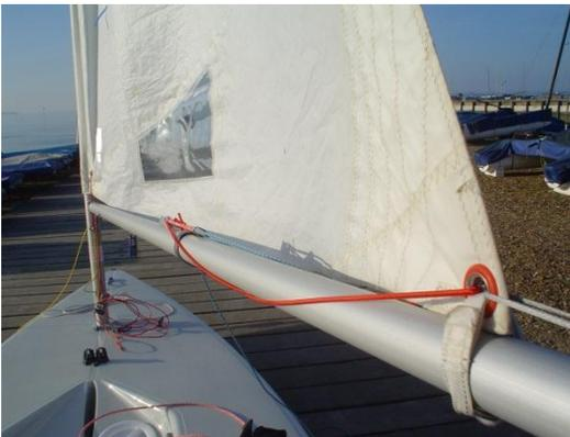
b. The line then returns under the boom on the other side and is tied off into the loop in the Elastic.
