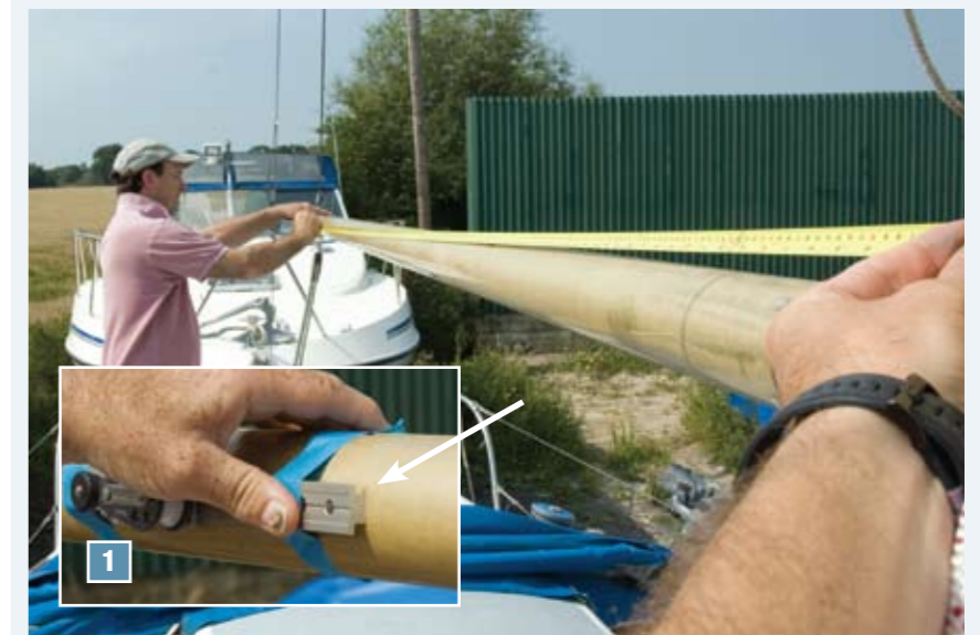
Step 1: Take measurements from the base of the mast slider to the eyelets – you could just put the sail on, and mark where the eyelets line up with the boom, but the sail will just get in the way if left on. This measurement gives the forward end of the track placement on the boom (inset arrow).
