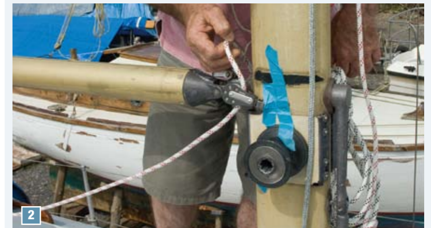
Step 1: Take measurements from the base of the mast slider to the eyelets – you could just put the sail on, and mark where the eyelets line up with the boom, but the sail will just get in the way if left on. This measurement gives the forward end of the track placement on the boom (inset arrow).
