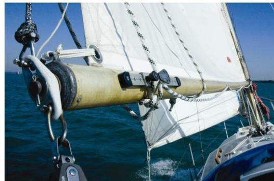
Lower the main halyard to the correct position for reefing and reef mainsail. If correct, mark the halyard at the position of the cleat with permanent marker.
