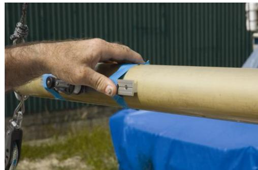
Remove track, drill using 4.2mm drill and tap using 5mm tap then secure in position using 5mm machine screw
