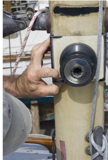
Use the bullseye as a template to mark the position of the two fixings with centre punch then, remove bullseye and drill using a 3.3mm drill before tapping using the 4mm tap. . After securing, the screws can be removed and the surplus length inside the boom cut off, to prevent possible snagging of internal control lines on the sharp ends of the screws.
