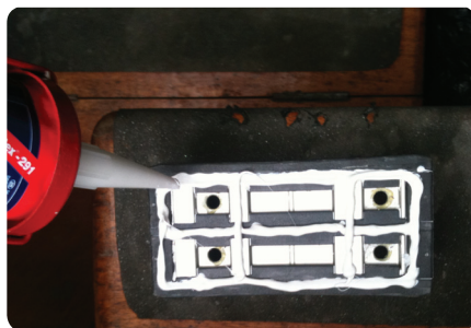
Adding sealant to the clutch base.
