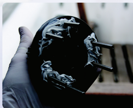
And also onto the bolt threads and winch base, be careful not to coat the winch gears though. The backing plate supplied is inserted inside and bolts are secured with M6 nyloc nuts.
