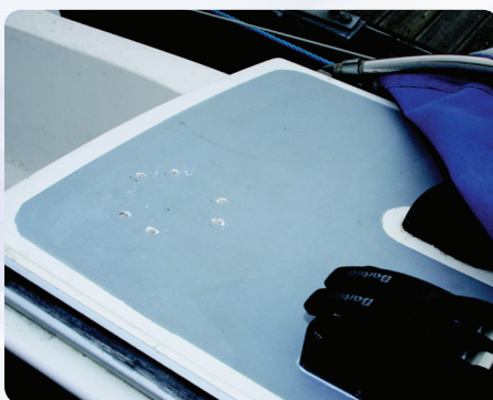
Insert sealant into the drilled holes.
