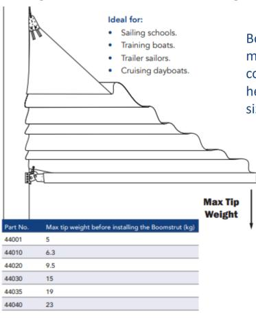
Boom tip weight should be measured with all sails, covers and lines fitted. This helps with getting the right size for your boat.
