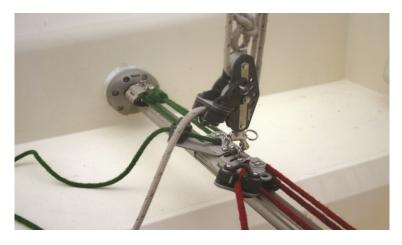
The Removable Track System is available in 3 sizes and can be used on yachts up to a maximum of 14.0m (46ft).
