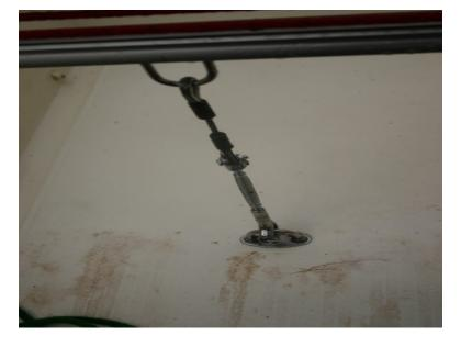
A similar construction with stainless steel wire and a U-Bolt secured in the cockpit floor can also be installed.
