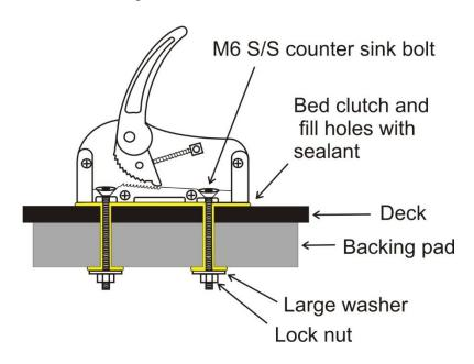
To ensure the best watertight seal is achieved, we would recommend slightly tightening the bolts, allow the sealant to cure for 24 hours and then tighten the bolts fully. This will allow the sealant to form a watertight gasket.
